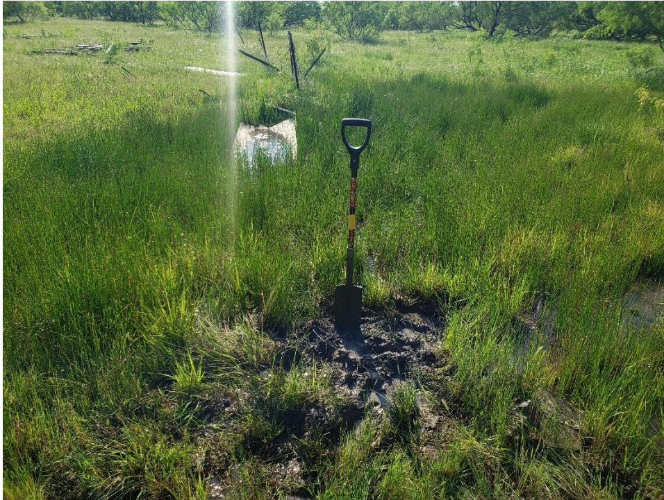
Photograph 27. View of WP 1. This sample location did not meet the three necessary criteria to be considered a wetland.
