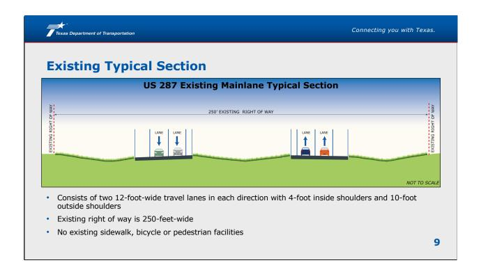
The existing roadway right of way is 250-feet-wide and consists of two 12-foot-wide travel lanes in each direction, northbound and southbound US 287. There is a 4-foot shoulder on the inside of both northbound and southbound lanes and a 10-foot outside shoulder on both sides. There are no existing sidewalk, bicycle or pedestrian facilities.
