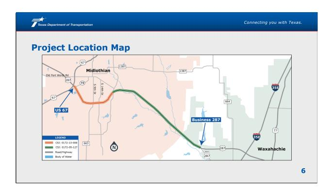
This project is for US 287 from US 67 to Business 287. The proposed improvements include constructing frontage roads in each direction with variable left-hand turn lanes and the addition of bicycle and pedestrian accommodations.
